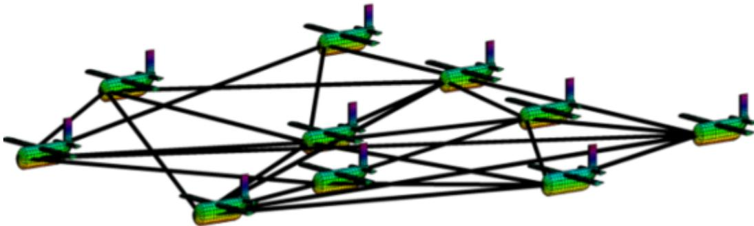
Dynamics network redesign provides an approach to improve the effectiveness of the human controllers' signal in reducing a wind gust perturbing the UAV swarm. Specifically, by rewiring the interaction network topology, we are able to amplify the human controllers' signals, to more effectively dampen the perturbation.
