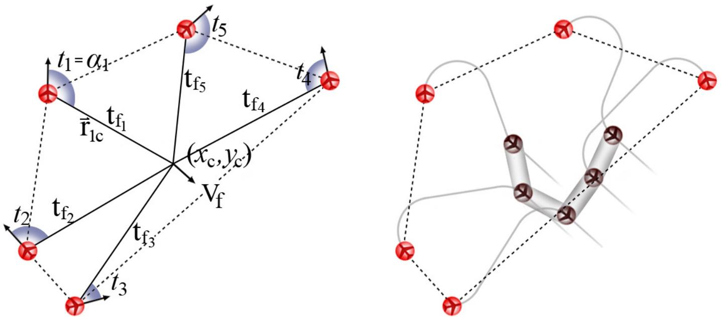
Optimization and Nonlinear-Programming methods are used to determine the shortest trajectories that bring the UAVs to a connected formation where they are in range of detection of one another and oriented in the same direction to maintain the connectivity. The methods are designed based on the fundamental concept of Pontryagin Minimum Principle (PMP) and bang-bang control.
