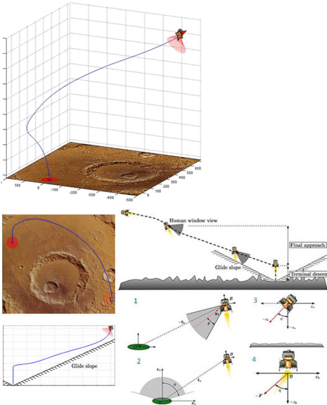
This problem considers a convex programming approach, based on model predictive control, for the numerical solution to a Mars powered-descent guidance problem in the presence of motion constraints. Specifically for the case of a Mars lander spacecraft, we consider the following constraints:
