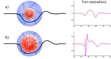
Fig. 4. (a) Avoiding the obstacle without entering protected zone (b) Turn rate increases dramatically when the UAV enters obstacle's protected zone
