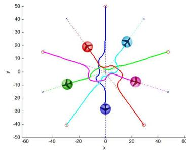
Fig. 11. Simulation trajectories when 5 vehicles fly through the same point
