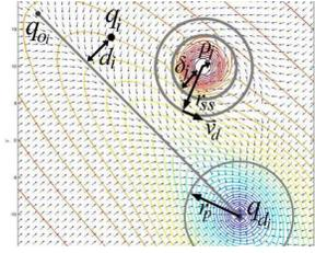
Fig. 3. The gradient vectors across the free configuration space
