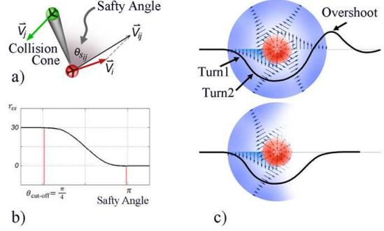
Fig. 7. (a) The collision cone and safety angle, (b) The plot of swirling radius adjusted by safety angle, (c) The overshoot disappears after swirling effect is dimmed down
