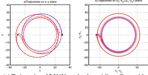
Fig. 8. (a) Trajectories of 2 UAVs under the swirling effects with 4 different initial headings (b) Trajectories on  $\bar{x}, \bar{y}$ -plane
