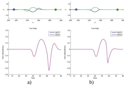
Fig. 10. Trajectory and turn rate of head-on case with  $r_{ss} = 30$ : (a) Swirling effect causes overshoots, (b) The overshoot disappears by safety angle method
