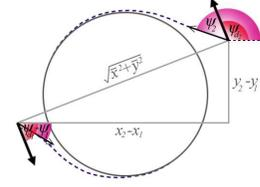
Fig. 9. The headings and desired heading of 2 vehicles under swirling effects when they in the course of collision
