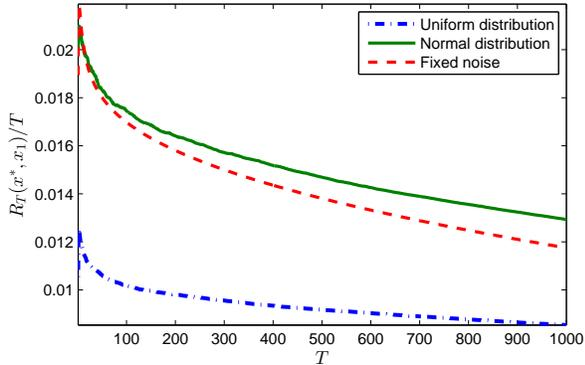
Figure 4. Regret performance for three different observation noise characteristics, where  $\mathcal{G}$  is a 100 node random 4-regular graph. The noise signals have been generated from distributions with mean  $-b_{\max}$  and standard deviation  $b_{\max}$ .
