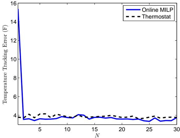
Fig. 2. Temperature tracking error of chilling load with online MILP and thermostat schedule for a month.
