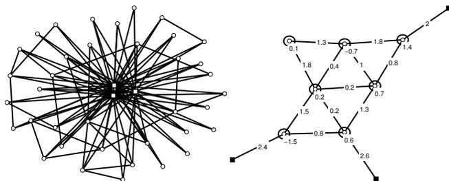
Fig. 3. (a) The resultant leader-follower network after applying **Protocol 1** to 10 spanning trees of the graph in Figure 2. (b) Reduced weighted agent graph corresponding to  $A_r$ ,  $B_r$  with leader agents (squares). Edges from an agent to itself (a self loop) are denoted by a circle around the agent.
